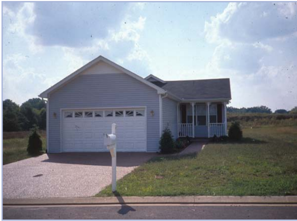
Garages must be recessed a minimum of 15' behind the front facade or porch.
